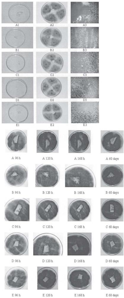
Fig. 2. The images of the control sample (1) and fungal growth (2) and detail (3, x18) after 72 h of inoculation: A-PU;B- PU/HC;C-PU/HC/KEL;D-PU/HC/KEL/CS;E-PU/HC/KEL/HA
